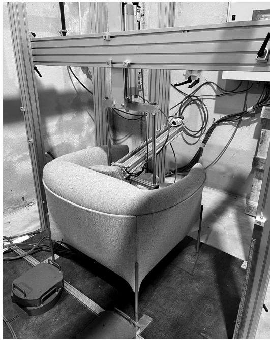
Fig. 03 Omnia endurance stress test in the lab.
